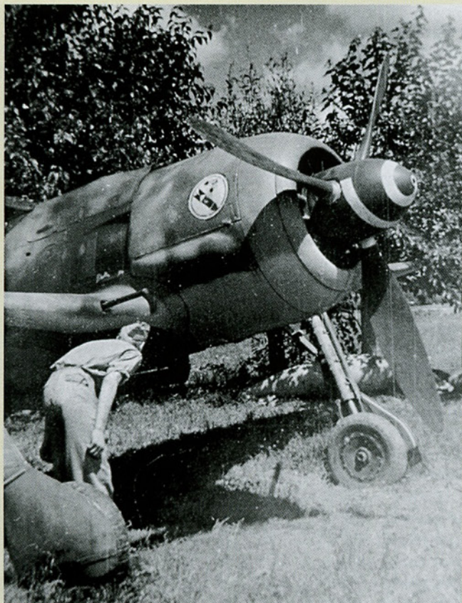
ABOVE: Ground crew of 1./SG 4 helping the pilot of 'White 2' strap in. Although this aircraft lacks head armour, a blown canopy and underwing bomb racks, it is thought that this is, in fact, an Fw 190 F-8, a version which was delivered to SG 4 in May 1944, shortly before the unit was withdrawn from the front due to its high losses. By this time the Luftwaffe's ground-attack units had phased out their earlier letter codes in favour of fighter-style markings.
